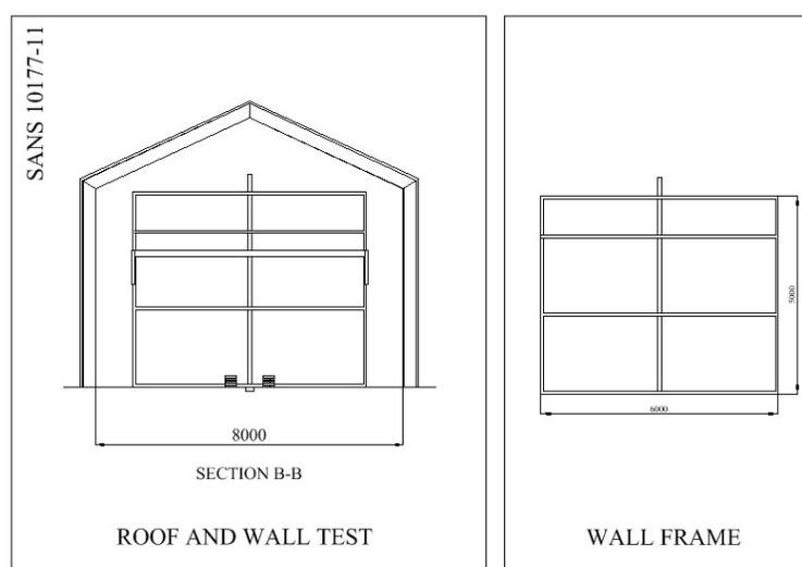
Figure 3: Typical side-cladding installation in SANS 10177 Part 11 facility
