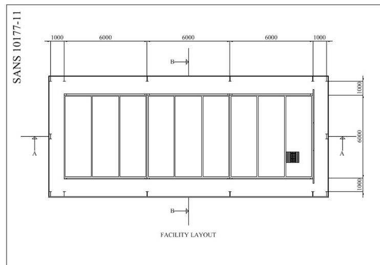
Figure 1: SANS 10177 test facility with specimen frames
